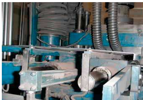
By changing over to the drylin® R linear plain bearing, the maintenance rate of this compaction unit could be extended by two years, despite high stressing from powder particles and abrasive agents.
