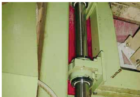
The machine now runs entirely free of troubles for multiple years with drylin® RJUM-01 linear bearings despite the extremely heavy – duty operation.
