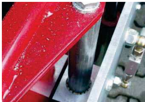
Saw mill: linear guide with iglidur® J plastic liner for the angle stops. iglidur® J liners are best suited for most linear applications due to their low wear and low friction properties.
