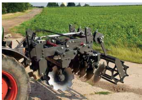
Since the sliding bearing should be maintenance-free, precise, compact, durable and very resilient, liners were mounted directly in the passages of the machine frame.
