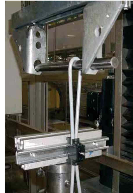
igus® tensile strength test with CFX clamps
